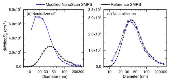
Fig. 6 PNSDs measured using the reference SMPS and modified NanoScan SMPS of (a) polydisperse NaCl aerosols without pre-conditioning and (b) polydisperse NaCl aerosols pre-conditioned with a neutralizer.
