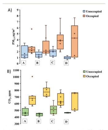
Fig. 5 Effect of occupancy on indoor PM<sub>2,5</sub> concentration (A) and CO<sub>2</sub> concentration (B): residences A-D were mechanically ventilated where residences A and B prohibited cooking, and residences C and D allowed cooking.
