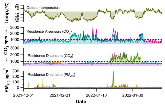
Fig. 11 Impact of outdoor temperature and ventilation on indoor pollutants  $CO_2$  and  $PM_{2.5}$  concentration. Impact of outdoor temperature and ventilation on indoor pollutants  $(CO_2)$  and  $PM_{2.5}$  concentration.
