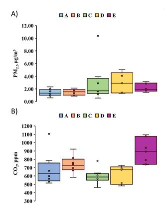
Fig. 6 Effect of MV (residence A–D) and NV (residence E) on indoor  $PM_{2.5}$  (A) and  $CO_2$  (B) concentration.
