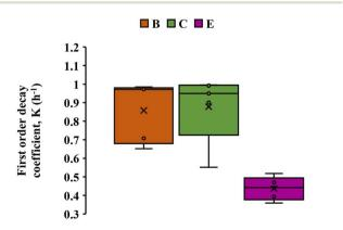
Fig. 7 First order decay coefficient (K) of PM<sub>2.5</sub> generated from five events of humidifier use in residence B, C, and E. Note that B and C employ MV, while E employs NV.
