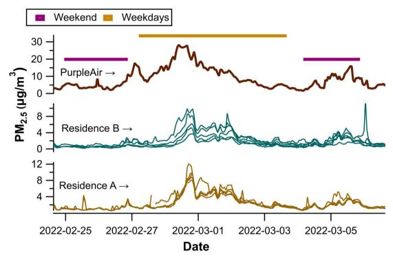
Fig. 10 Hourly variations of indoor PM<sub>2.5</sub> level with outdoor PM<sub>2.5</sub> level, during weekdays and weekends. The outdoor PurpleAir data was treated with corrections recommended by the US EPA.82
