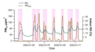
Fig. 8 Effect of humidifier on indoor PM<sub>2.5</sub> emission. Data from one sensor is shown here as a case study
