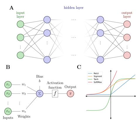
Fig. 2 Neural network and its building blocks. (A) Schematic of a NN model with an input layer (green), N hidden layers (blue) and an output layer (red). (B) Illustration of a node inside the hidden layers. Bottom right (C): examples of common activation functions.
