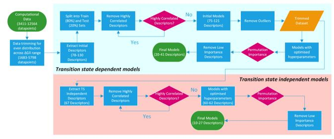
Overview of the machine learning model generation process, from computational data to final models.
