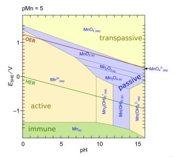
Fig. 1 Potential-pH (Pourbaix) diagram of Mn calculated using MEDUSA<sup>27</sup> at an activity of dissolved species of 10<sup>-5</sup>. Shading color of the areas refers to the water solubility of the respective phase: green - insoluble metal; blue - insoluble oxide/hydroxide, yellow - soluble ion. Red and green lines indicate oxidation/reduction potentials of water to molecular oxygen and hydrogen, respectively.
