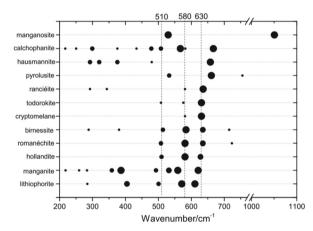
Fig. 3 Raman band positions of selected MnO<sub>x</sub>. The dot size is proportional to the observed band intensities. Figure reprinted from ref. 41 with permission. Copyright 2019 John Wiley & Sons, Ltd.
