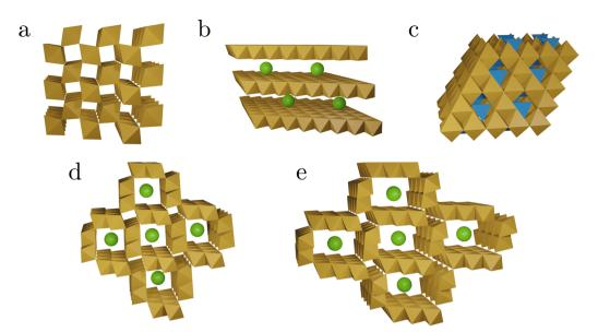
Fig. 2 Schematic representations of the tunnel and layer structures in MnO<sub>x</sub> discussed in this work. The structures shown consist of MnO<sub>6</sub> octahedra (brown),  $MnO_4$  tetrahedra (blue), and spheres representing other cations or water (green). Structural details are listed in Table 1. Pyrolusite,  $\beta$ -MnO<sub>2</sub> (a), birnessite  $\delta$ -MnO<sub>2</sub> (b), spinel structure (c), hollandite  $\alpha$ -MnO<sub>2</sub> (d), and romanechite (e).
