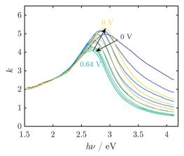
Fig. 5 UV/Vis spectra of thin MnO<sub>x</sub> films, represented by the imaginary part k of the complex refractive index, at pH 13 during electrochemical cycling show reversible peak shifts. In this example, the OER onset was observed at ≈0.55 V vs. Ag/AgCl/3 M KCl. Figure adapted from ref. 32 under CC BY 3.0 license.
