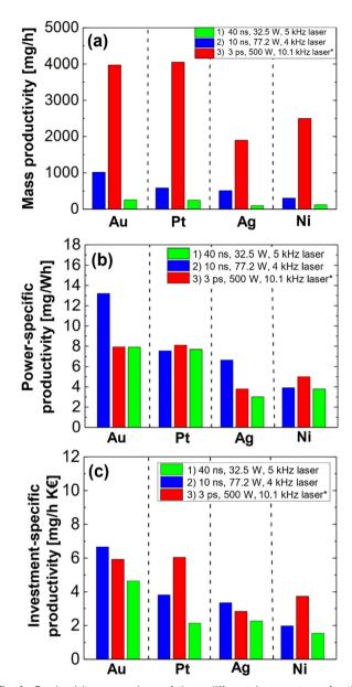
Fig. 4 Productivity comparison of three different laser systems for the ablation of Au, Pt, Ag, and Ni in water, adapted from ref. 115 with permission from author, licensed under CC BY 4.0, copyright 2018. Each figure indicates a different productivity calculation approach: (a) mass productivity, (b) power-specific productivity, and (c) investment-specific productivity. The asterisk (\*) indicates that the data is reproduced from ref. 52 with permission from IOP Publishing Ltd, copyright 2016.
