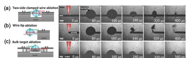
Fig. 11 Bubble morphology depending on the target geometry of (a) wire target clamped on both ends, (b) wire target clamped on one end, and (c) bulk target. Adapted from ref. 100 with permission from the PCCP Owner Societies, copyright 2016.
