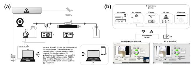
Fig. 17 Remote monitoring and controlling system. (a) Schematic representation of the system configuration, (b) controlled devices with in-site PC and the screenshot of off-site controlling devices. Adapted from ref. 166 with permission from AIP Publishing, copyright 2019
