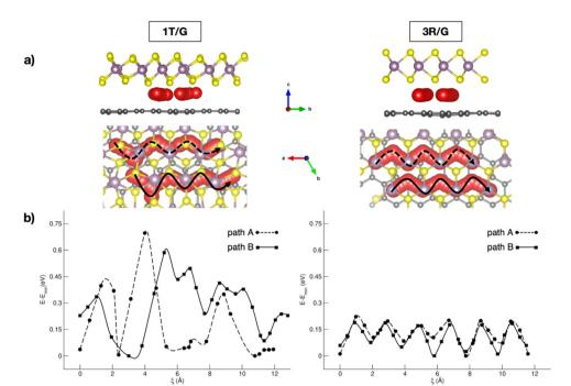
Fig. 1 (a) Side and top views of Na migration pathways through 1T- and 3R-MoS<sub>2</sub>/G interfaces; (b) corresponding energetics computed with the CI-NEB method at the PBE-D3BJ level of theory. Reproduced from ref. 76 [A. Massaro et al., J. Phys. Chem. C, 2021, 125, 2276–2286]. Copyright 2021 American Chemical Society.76
