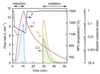
**Fig. 3** Time evolution of the temperature, reactor pressure, and flow rates of the gas products (O<sub>2</sub>, CO, and H<sub>2</sub>) during a representative redox cycle using an alveolar foam of CeO<sub>2</sub> (18.1 kg) and with a mean  $P_{\rm solar}$  = 42.0  $\pm$  6.2 kW. Reproduced with permission from ref. 17 with permission from Elsevier.
