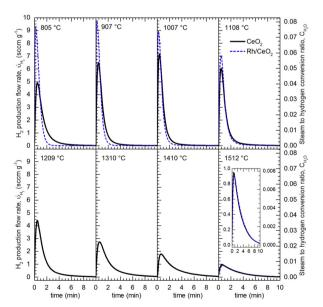
Fig. 7 Hydrogen release profiles obtained by water splitting at different temperatures (flow of 278 sccm of 20% H<sub>2</sub>O in Ar) over CeO<sub>2</sub> (Black lines) and Rh/CeO2 (Dashed blue lines) previously reduced in Ar at 1488 °C. Reproduced with permission from ref. 56 with permission from Elsevier.
