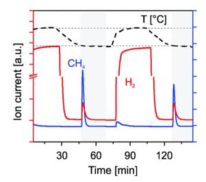
Fig. 8 Formation of hydrogen and methane at 500 °C from water (flow of 278 sccm of 20%  $\rm H_2O$  in Ar) and carbon dioxide by reoxidation of Rh/CeO<sub>2</sub> previously reduced in  $\rm H_2/Ar$  at 500 °C rhodium-doped ceria. Reproduced with permission from ref. 94 with permission from RSC.
