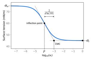
Fig. 2 Illustration of the Sigmoid model (blue solid line, eqn (25)) with parameters  $\sigma_{\rm w}$  = 75 mN m<sup>-1</sup>,  $\sigma_i$  = 45 mN m<sup>-1</sup>, p = -4, and d = 0.869. The critical micelle concentration "CMC" is estimated by intersecting the tangent line at the inflection point with a horizontal line at  $\sigma(x_i \to \infty)$ .
