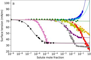
Fig. 6 Surface tension fits with the Sigmoid model for all tested substances (A) on a linear x-axis scale (B) on a logarithmic x-axis scale.
