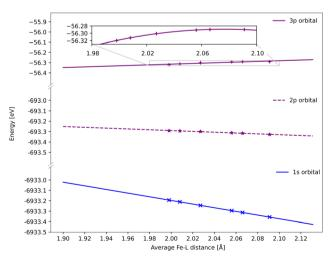
Fig. 10 DFT BP86 orbital energies of the 1s, 2p and 3p orbitals along the GS minimum -  $^3MC$  minimum coordinate for the  $^3MC$  state. For the porbitals the energy is an average of all three orbitals with the same principal quantum number. Linear regressions give gradients of -1.76 eV Å<sup>-1</sup> for 1s, -0.39 eV Å<sup>-1</sup> for 2p, and 0.34 eV Å<sup>-1</sup> for 3p, although the 3p orbital energies deviate from linear behavior (see inset).
