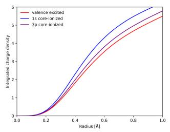
Fig. 8 Integrated RAS radial charge density (RCD) plots of the <sup>3</sup>MC valence state, and the corresponding states with 1s and 3p holes calculated at the <sup>3</sup>MC equilibrium geometry. To avoid effects of changes in core orbital occupation, only the Fe 3d  $t_{2q}$  and  $e_q$  orbitals were included. Radial spin densities (RSD) for the same states are shown in Fig. S17 (ESI†).
