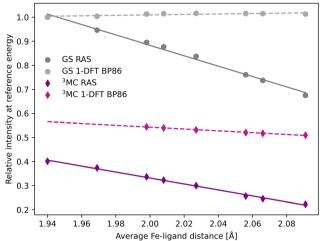
Fig. 5 Emission intensities at the GS Kβ maximum energy 7057.9 eV for XES spectra in Fig. 3 plotted as a function of the Fe-ligand distance. Linear regression lines were fitted for each set of calculations.
