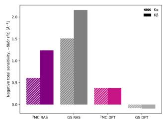
Fig. 7 Sensitivity of K $\beta$  and K $\alpha$  to changes in the Fe-ligand distance, shown as the negative value of the total sensitivity  $(-\delta I/\delta r)$  at the GS emission maximum energy (6404.3 eV for Kα and 7057.9 eV for Kβ).
