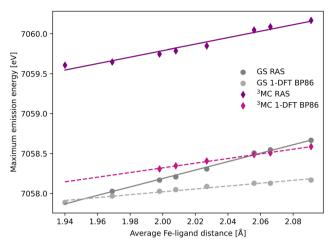
Fig. 4 Energies of the Kβ emission maxima for spectra in Fig. 3 plotted as a function of the Fe-ligand distance. Linear regression lines were fitted for each set of calculations.
