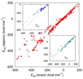
Fig. 11 Comparison of the leading order covalent  $(E_{xc})$ , ionic  $(E_{cl})$ , and total interaction energies ( $E_{int}$ ) with their exactly computed values for a set of over 800 different compounds covering several types of bonding regimes. Taken from ref. 228, where more details can be found, with permission granted by the retained rights of the authors. Data are provided in kcal  $mol^{-1}$
