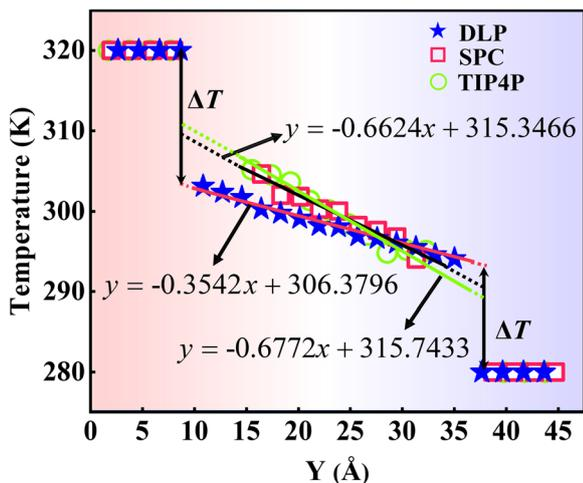
Fig. 8 The temperature distributions along the  $y$  direction calculated from dynamical simulations with DLP and empirical potentials. The  $x$  in the function expression represents the position in the  $y$ -direction, and  $y$  on behalf of temperature.
