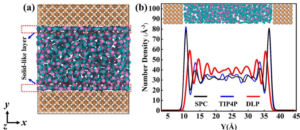
Fig. 6 (a) The thermal equilibrated structures of water layers near the solid wall obtained by dynamical simulations and (b) water density profiles along the  $y$  direction calculated from dynamical simulations with different potentials.
