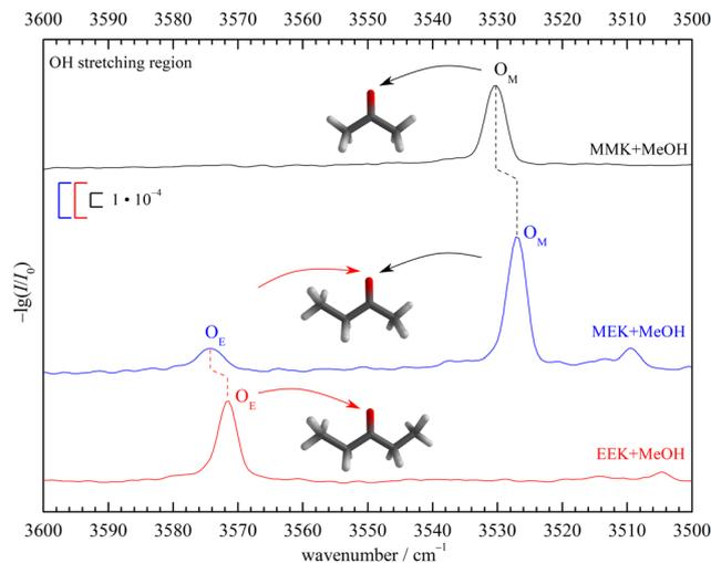
Fig. 2 Jet FTIR OH-stretching spectra of MEK, EEK and MMK<sup>45</sup> (scaled intensity) co-expanded with MeOH. Dashed lines connect analogous docking sites and lead to an unambiguous experimental assignment and preference for methyl side oxygen docking ( $O_M$ ) over ethyl side docking ( $O_E$ ) of MeOH to MEK. See Fig. S7 in the ESI† for more details.
