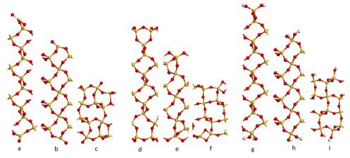
Fig. 2 Side view of the cleaved (C) (a-c) containing 39, 39 and 36 atomic layers respectively), reconstructed (R) (d-f) and hydroxylated (H) (q-i) α-SiO<sub>2</sub> surfaces. (a, d and g) (001), (b, e and h) (100) and (c, f and i) (101)  $\alpha$ -SiO<sub>2</sub> surfaces, respectively. Atoms are coloured Si: yellow and O: red. <sup>27,29–31,33,34,54–56</sup>
