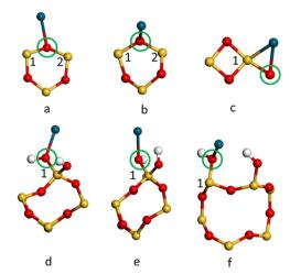
Fig. 5 The geometries of the optimal adsorption sites of Pd(g) on the 2  $\times$  $3 \times 1$  (a) R(001), (b) R(100), (c) R(101) and hydroxylated (d) H(001), (e) H(100) and (f) H(101)  $\alpha$ -SiO $_2$  slabs. In each case, the local environment of the adsorbed Pd atom and the surface siloxane ring is shown looking side on to the slab with other atoms removed for clarity. Atoms are coloured Si: vellow. Pd: dark blue. O: red and H: white
