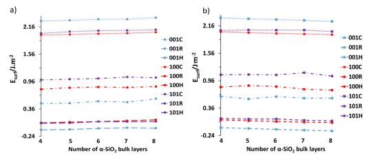
Fig. 3 (a) The surface energies of the 4 to 8 layered cleaved (C), reconstructed (R) and hydroxylated (H) α-SiO<sub>2</sub> surfaces at the PBE level of theory, and (b) the cleaved (C) reconstructed (R) and hydroxylated (H)  $\alpha$ -SiO<sub>2</sub> surfaces with TS dispersion corrections included (PBE-TS)
