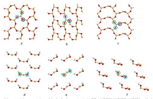
Fig. 4 The top view of the extended representations of the  $1 \times 1 \times 1$  reconstructed  $\alpha$ -SiO<sub>2</sub>, (a) R(001), (b) R(100), (c) R(101) and hydroxylated (d) H(001), (e) H(100) and (f) H(101) slabs and the possible Pd<sub>1</sub> adsorption sites on each surface. Colours are used to identify sites with site "a": green, site "b": indigo and site "c" dark blue. Atoms are coloured Si: yellow, O: red and H: white. Only the topmost atoms in each case are shown for clarity.
