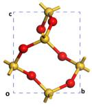
Fig. 1 The periodic  $Si_3O_6$  bulk of crystalline  $\alpha\text{-SiO}_2$  as calculated with PBE-TS ( $a = b = 4.98 \text{ Å}, c = 5.40 \text{ Å}, \alpha = \beta = 90^{\circ}, \gamma = 120^{\circ}$ ). Cell vector a is into the page, label "o" marks the origin of coordinates. Atoms are coloured Si: yellow and O: red.
