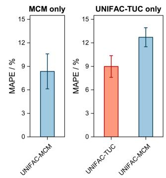
Fig. 3 Mean Absolute Percentage Error (MAPE) of the predicted mole fraction of the low-boiling component in the vapor phase in VLE with UNIFAC-MCM for the systems that can only be modeled by UNIFAC-MCM (left, 'MCM only', 9 systems), and those systems that can also be predicted with UNIFAC-TUC but not with UNIFAC (middle, 'UNIFAC-TUC only', 169 systems). Error bars denote standard errors of the means.
