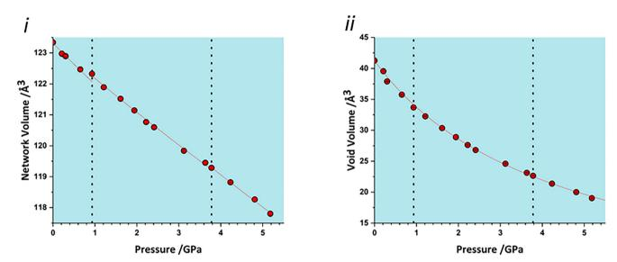
Fig. 5 i) Network volumes at increasing pressure. ii) Void volumes at increasing pressure. Dashed lines in all plots represent phase transitions based on this work and that of Holanda et al.
