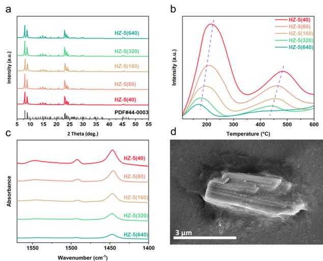
**Fig. 1** (a) XRD patterns of HZSM-5 zeolites; (b)  $\text{NH}_3$ -TPD curves of HZSM-5 zeolites; (c) Py-IR spectra of HZSM-5 zeolites recorded after the removal of weakly adsorbed pyridine by evaporation at 200 °C; (d) SEM diagram of HZ-5(40).
