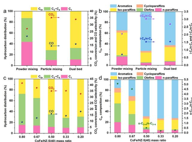
Fig. 3 Hydrocarbon distribution (a) and C<sub>5+</sub> composition (b) in the case of CO<sub>2</sub> hydrogenation over CoFe/HZ-5(40) with different proximities; hydrocarbon distribution (c) and C<sub>5+</sub> composition (d) of CO<sub>2</sub> hydrogenation over tandem catalysts with different CoFe/HZ-5(40) mass ratios. Reaction conditions: 320 °C, 3.0 MPa, H<sub>2</sub>/CO<sub>2</sub>/N<sub>2</sub> = 72/24/4 (vol%), 4000 mL g<sub>cat.</sub><sup>-1</sup> h<sup>-1</sup>, time on steam = 14 h.
