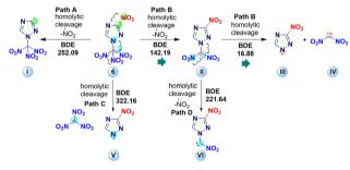
Fig. 7 Proposed thermal decomposition pathway for compound  $\bf 6$  (BDEs are given in kJ mol<sup>-1</sup>).
