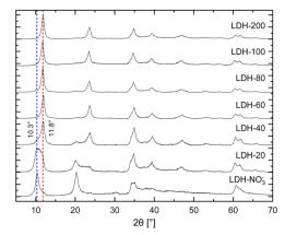
Fig. 1 PXRD patterns of pristine LDH-NO $_3^-$  and the anion exchanged samples LDH-A (A=20, 40, 60, 80, 100 and 200 standing for the initial carbonate concentration in mmol L $^{-1}$  in the anion exchange solution). The NO $_3^-$ - and CO $_3^{2-}$ -intercalated phases can be identified by the characteristic basal reflections at 10.3 and 11.8° 2 $\theta$ , respectively.
