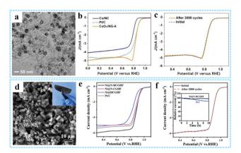
Fig. 15 (a) TEM image of the CoO<sub>x</sub>/NG-A composite. (b) ORR polarization curves of  $CoO_x/NG-A$  at 10 mV s<sup>-1</sup> and 1600 rpm. (c) Cycling performance of CoO<sub>x</sub>/NG-A. Reprinted with permission from ref. 51. Copyright 2017 American Chemical Society. (d) Top-view SEM image of Ni@N-HCGHF. (e) LSV curves for the ORR of various samples. (f) Cycling performance of Ni@N-HCGHF over 2000 CV cycles. Reproduced with permission from ref. 121 Copyright 2020 Wiley-VCH.
