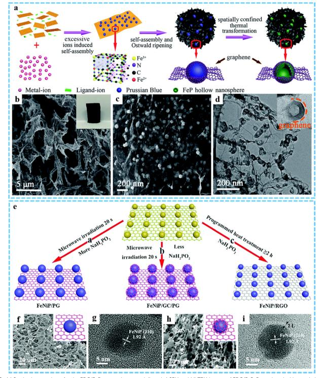
Fig. 7 (a) Synthesis procedures for the 3DG/FeP composite aerogel. (b and c) SEM and (d) TEM images of 3DG/FeP. Reproduced with permission from ref. 101. Copyright 2020 Royal Society of Chemistry. (e) Schematic of the synthetic process of FeNiP/PG, FeNiP/GC/PG and FeNiP/RGO composites. (f) SEM and (g) HRTEM images of FeNiP/PG. (h) SEM and (i) HRTEM images of FeNiP/GC/PG. Reproduced with permission from ref. 82. Copyright 2019 Royal Society of Chemistry.
