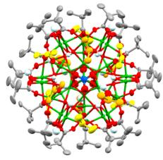
Fig. 2 Solid-state structure of  $Cu_{31}$ -oxo cluster 4. Cu = green, O = red, C = grey, N = blue, H = very pale blue (non-coordinated/H-bonded PrOH Cs = yellow, coordinated PrOH Cs = orange). Ellipsoids displayed at 50% and hydrogen atoms (except OH) omitted.
