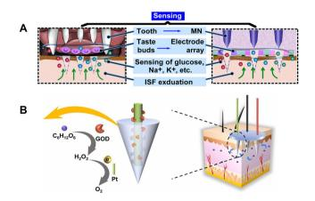
Fig. 13 Integration of MNs for sampling and glucose sensing. (A) Illustration of transdermal sensing of an MN theranostic platform. Adapted with permission from ref. 169. Copyright 2022, American Association for the Advancement of Science. (B) Working mechanism of wire electrode-embedded MN patches. Adapted with permission from ref. 170. Copyright 2022, Elsevier.
