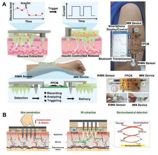
Fig. 5 ISF collection by iontophoresis through porous and solid MNs. (A) A closed-loop system based on mesoporous MN-RI for diabetes treatment. Adapted with permission from ref. 75. Copyright 2021, Wiley-VCH. (B) A touch-actuated glucose sensor fully integrated with solid MNs and RI for diabetes monitoring. Adapted with permission from ref. 22. Copyright 2022, Elsevier.
