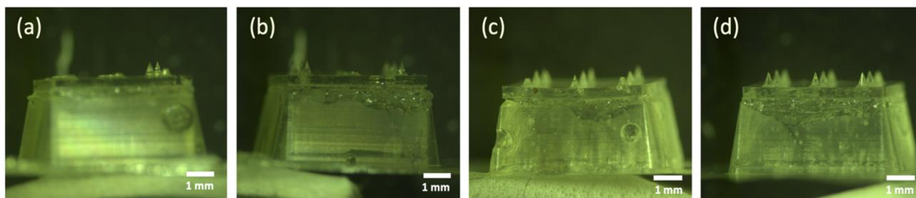
**Fig. 2** Representative microscopic images of fabricated empty dMNAs using the automatic dispensing system. Empty dMNAs were produced with (a) 2% (w/v), (b) 3% (w/v), (c) 4% (w/v), and (d) 5% (w/v) trehalose/pullulan ( $n = 3$ ). The weight ratio of trehalose to pullulan was 50 : 50.
