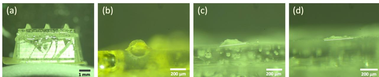
**Fig. 4** (a) The fabricated WIV dMNA with 100% of intact microneedles. WIV loaded microneedles after (b) 2 minutes, (c) 5 minutes, and (d) 10 minutes of skin dissolution. The shape of the intact microneedle before dissolution was similar to that in Fig. 3b. Longer dissolution times were not evaluated as the leftover volume after 10 minutes was sufficiently low.
