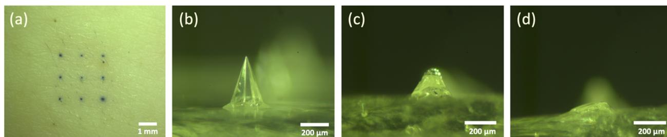
**Fig. 3** Representative microscopic images of skin penetration and dissolution tests of empty dMNAs ( $n = 3$ ). (a) Human abdominal skin *ex vivo* penetrated with a 5% (w/v) trehalose/pullulan  $3 \times 3$  dMNA. (b)–(d) Microneedle made of 5% (w/v) trehalose/pullulan (b) before skin dissolution and leftover microneedle (c) after 15 minutes and (d) after 30 minutes of skin dissolution.
