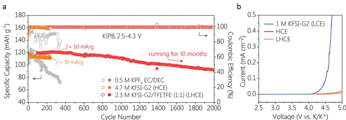
**Fig. 1** (a) Cycling performance of K|PB batteries in 0.5 M KPF<sub>6</sub> EC DEC electrolyte at  $50 \text{ mA g}^{-1}$ , HCE at  $10 \text{ mA g}^{-1}$ , and LHCE at  $50 \text{ mA g}^{-1}$ . (b) LSV of various concentrations of KFSI/G2 electrolytes in K|Al coin cells with Al as the working electrode and K metal as the counter electrode. The scan rate is  $0.5 \text{ mV s}^{-1}$ .
