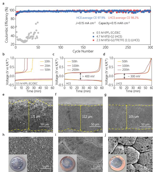
**Fig. 3** (a) Cycling performances of K|Cu coin cells and the corresponding voltage profiles in (b) 0.5 M KPF<sub>6</sub> EC/DEC electrolyte, (c) HCE and (d) LHCE at 0.15 mA cm<sup>-1</sup>. (e–g) Cross-sectional and (h–j) top-view SEM images of K deposition morphologies in (e and h) 0.5 M KPF<sub>6</sub> EC/DEC, (f and i) HCE and (g and j) LHCE. Optical images of K deposits on Cu foil are shown in the inset of h–j. The capacity of K metal on the Cu substrate was 4.0 mA h cm<sup>-2</sup>.
