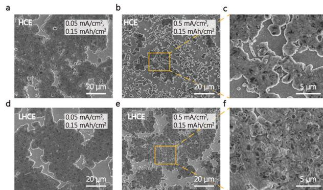
**Fig. 4** Top-view SEM images of K deposition morphologies in (a–c) HCE and (d–f) LHCE with enlarged views (c and f) at a current density of (a and d) 0.05 mA cm<sup>-2</sup> and (b and e) 0.5 mA cm<sup>-2</sup> with a capacity of 0.15 mA h cm<sup>-2</sup>.
