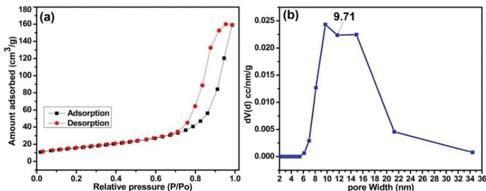
Fig. 4 BET result of MAFPA: (a)  $\text{N}_2$  adsorption–desorption isotherm and (b) pore size distribution.
