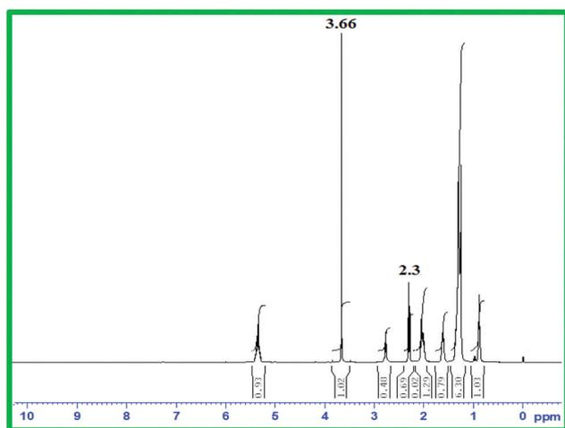
Fig. 13 <sup>1</sup>H NMR of soybean oil biodiesel.
