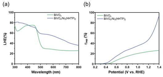
Fig. 5 (a) Light harvesting efficiency (LHE) (%) and (b) charge separation efficiency (η<sub>sep</sub>) of BiVO<sub>4</sub> and BiVO<sub>4</sub>/Ni<sub>3</sub>(HHTP)<sub>2</sub>.
