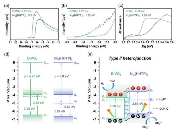
Fig. 4 UPS of BiVO<sub>4</sub> and BiVO<sub>4</sub>/Ni<sub>3</sub>(HHTP)<sub>2</sub> for obtaining (a) work function (f) and (b) VBM. (c) UV-vis spectra of BiVO<sub>4</sub> and BiVO<sub>4</sub>/Ni<sub>3</sub>(HHTP)<sub>2</sub>. Schematic energy band diagram of BiVO<sub>4</sub> and BiVO<sub>4</sub>/Ni<sub>3</sub>(HHTP)<sub>2</sub> (d) before contact and (e) after contact.
