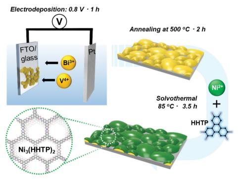
Fig. 1 Schematic diagram of the synthesis process for the BiVO<sub>4</sub>/Ni<sub>3</sub>(HHTP)<sub>2</sub> heterostructure on FTO/glass substrate.
