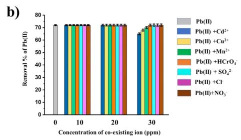
Fig. 11 (a) Effect of co-existing ions on Cr(vi) removal by GO@Zn-Hap@CA. (b) Effect of co-existing ions on Pb(II) removal by GO@Zn-Hap@CA.
