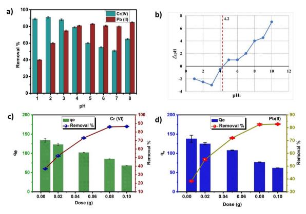
Fig. 6 (a) Effect of pH on Cr(vi) and Pb(ii) adsorption (initial metal concentration 100 ppm, dose 0.05 g; contact time:100 minutes); (b) point of zero charge graph of GO@Zn-Hap@CA; (c) effect of dose on Cr(iv) adsorption; (d) effect of dose on Pb(ii) adsorption (pH 2 = Cr(vi) and pH 5 = Pb(ii), initial metal concentration of 100 ppm, contact time of 100 minutes).
