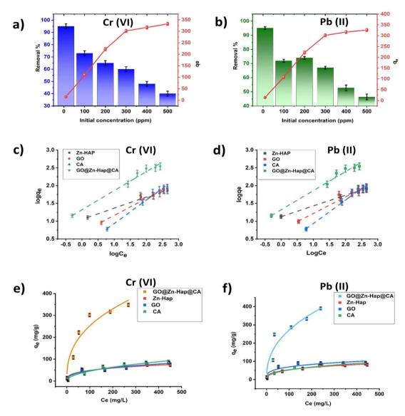
Fig. 7 Effect of the initial Cr(vı) (a) and Pb(II) (b) concentrations on the adsorption capacity and removal efficiency. Linear fitting of the Freundlich isotherm for Cr(v) (c) and Pb(II) (d). Non-linear fitting of the Freundlich isotherm for Cr(vI) (e) and Pb(II) (f) of Zn-Hap, GO, CA and GO@Zn-Hap@CA; (pH 2 = Cr(vi)) and pH 5 = Pb(ii), dose 0.05 g; contact time: 100 minutes).
