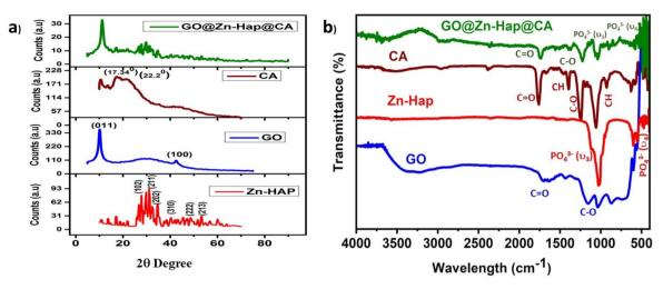
Fig. 1 (a) XRD pattern of Zn-Hap, GO, CA, and GO@Zn-Hap@CA; (b) FTIR analysis of GO, Zn-Hap, CA, and GO@Zn-Hap@CA.
