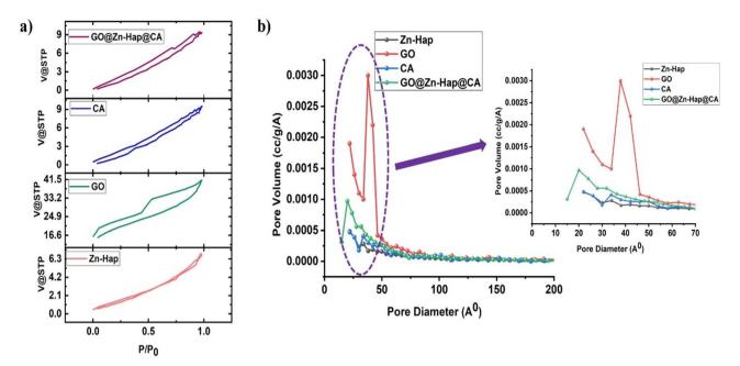
(a) N<sub>2</sub> adsorption desorption isotherms, (b) BJH adsorption pore size distribution for GO, Zn-Hap, CA membrane and GO@Zn-Hap@CA.
