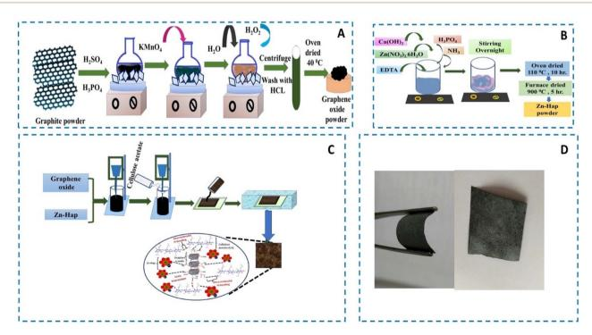
Scheme 1 Synthesis of GO (A); synthesis of Zn-Hap (B); preparation of GO@Zn-Hap@CA composite membrane (C); digital photograph of GO@Zn-Hap@CA (D).
