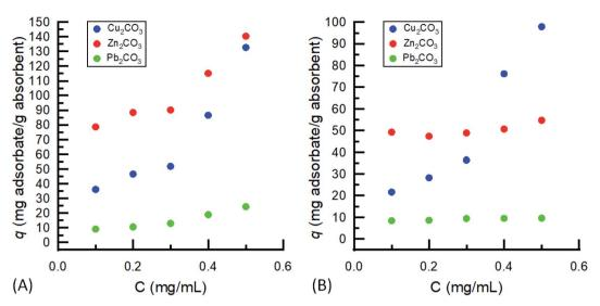
Fig. 6 Concentration dependent adsorption for removal of adsorbate ((●) Cu(II), (●) Zn(II), and (●) Pb(II)) at time 120 minutes by (A) 2.0 wt% and (B) 0.2 wt% carbon nanomaterial (CNM)-based aerogels.
