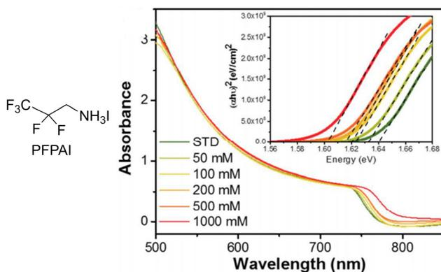
Fig. 31 UV-Vis spectra showing the tuning of the band gap upon passivation with different concentrations of PFPAl.<sup>131</sup> Reproduced with permission from ref. 131. Copyright 2018, American Chemical Society.
