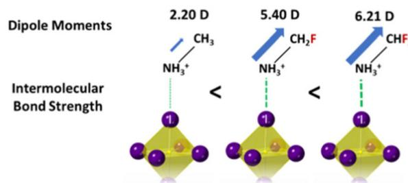
Fig. 4 The order of strengthening of the hydrogen bond between the A-site cation and the metal halide lattice due to the dipolar effect of fluorine.<sup>17</sup> Reproduced with permission from ref. 17. Copyright 2020, American Physical Society.
