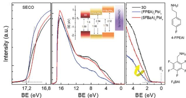
Fig. 23 UPS spectra and valence and conduction band energies of pristine 3D, 4-FPEAI and  $F_3$ BAI passivated perovskites.<sup>12</sup> Reproduced with permission from ref. 12. Copyright 2020, John Wiley and Sons.
