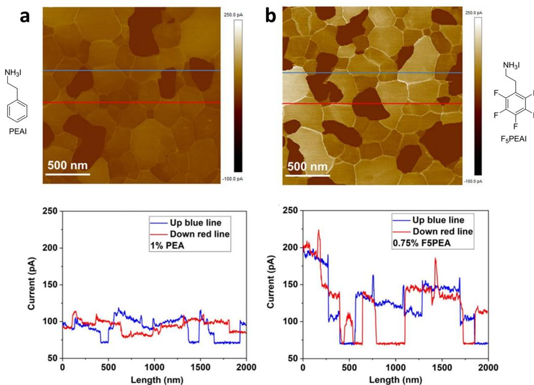
Fig. 22 (a) c-AFM studies of the 1%-PEAI-based bilayer perovskite. (b) c-AFM studies of the 0.75% F<sub>5</sub>PEAI and 0.25% PEA I-based bilayer perovskite.<sup>39</sup> Reproduced with permission from ref. 39. Copyright 2020, John Wiley and Sons.
