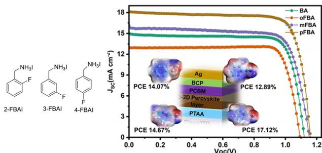
Fig. 11  $J$ - $V$  curve confirming the best performance for the (4-FBA) $_2$ -MA $_4$ Pb $_4$ I $_{16}$  PV device in an inverted configuration.<sup>73</sup> ESPs are shown in the inset (unit a.u.). Reproduced with permission from ref. 73. Copyright 2022, American Chemical Society.
