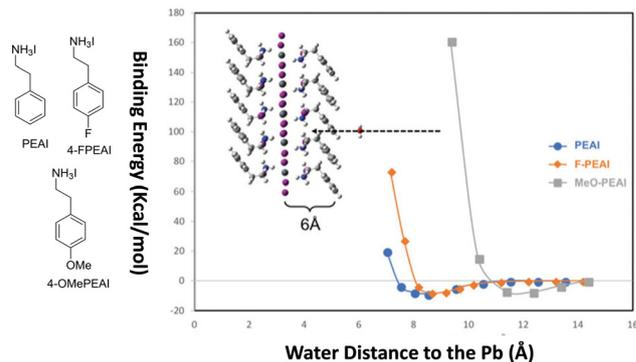
Fig. 14 Plots for theoretically calculated binding energy vs. water distance from the Pb layer for the RP-perovskites based on PEAI, 4-FPEAI, and 4-OMePEAI spacers.<sup>64</sup> Reproduced with permission from ref. 64. Copyright 2019, John Wiley and Sons.
