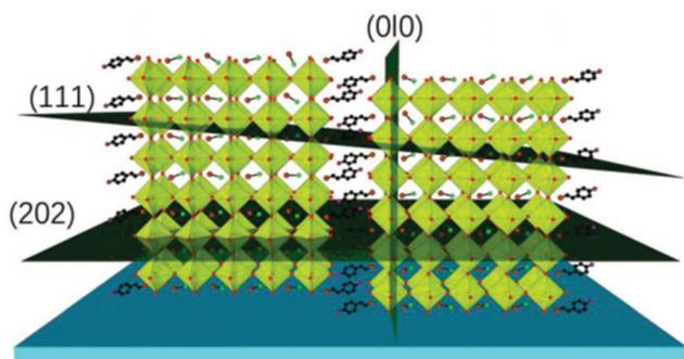
Fig. 9 Crystal growth along the (202) and (111) planes of  $(4\text{-FPEA})_2\text{MA}_4\text{Pb}_5\text{I}_{16}$ .<sup>60</sup> Reproduced with permission from ref. 60. Copyright 2019, John Wiley and Sons.
