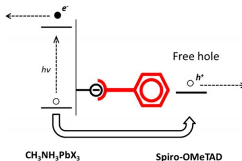
Fig. 29 Passivation of X<sup>-</sup> centres present towards the surface of the perovskite film or crystal with IPFB.<sup>36</sup> Reproduced with permission from ref. 36. Copyright 2014, American Chemical Society.
