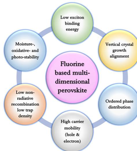
**Fig. 5** Tailoring of optoelectronic properties and stability by exploration of fluorinated spacers or passivators.<sup>100</sup>
