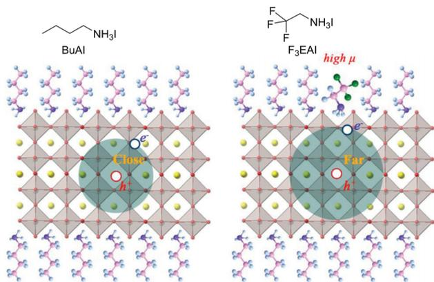
Fig. 17 The lattice polarization imparted by the  $F_3EAI$  spacer offering exciton screening and lower binding energy.<sup>124</sup> Reproduced with permission from ref. 124. Copyright 2018, John Wiley and Sons.
