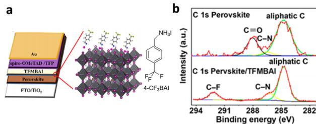
Fig. 28 (a) The passivation of the triple cation perovskite with 4-CF<sub>3</sub>BAI. (b) XPS spectrum showing disappearance of the C=O peak upon passivation.<sup>130</sup> Reproduced with permission from ref. 130. Copyright 2021, American Chemical Society.
