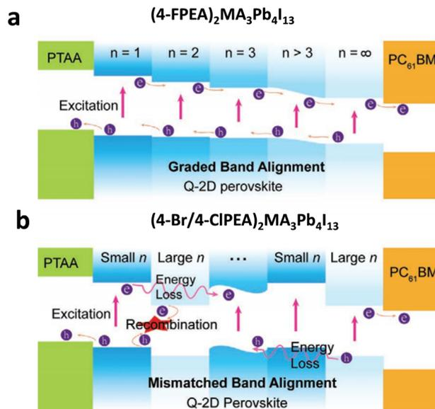
Fig. 13 (a) Suitable band alignment due to gradient phase distribution in  $(4\text{-FPEA})_2\text{MA}_3\text{Pb}_4\text{I}_{13}$ . (b) Carrier trapping due to random phase distribution in  $(4\text{-Br}/4\text{-ClPEA})_2\text{MA}_3\text{Pb}_4\text{I}_{13}$ .<sup>101</sup> Reproduced with permission from ref. 101. Copyright 2020, John Wiley and Sons.
