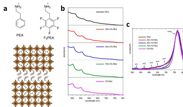
Fig. 15 (a) RP-perovskite with 1:1 PEA: $\text{F}_5\text{PEA}$  cations. (b) UV-Vis and PL spectra reveal the presence of mixed-dimensional phases with  $n = 1, 2, 3, 4$ , etc. upon 25–75% replacement of PEA with the  $\text{F}_5\text{PEA}$ -based spacer. (c) PL spectrum obtained from the front excitation revealing the highest intensity of the 3D-phase.<sup>62</sup> Reproduced with permission from ref. 62. Copyright 2019, American Chemical Society.
