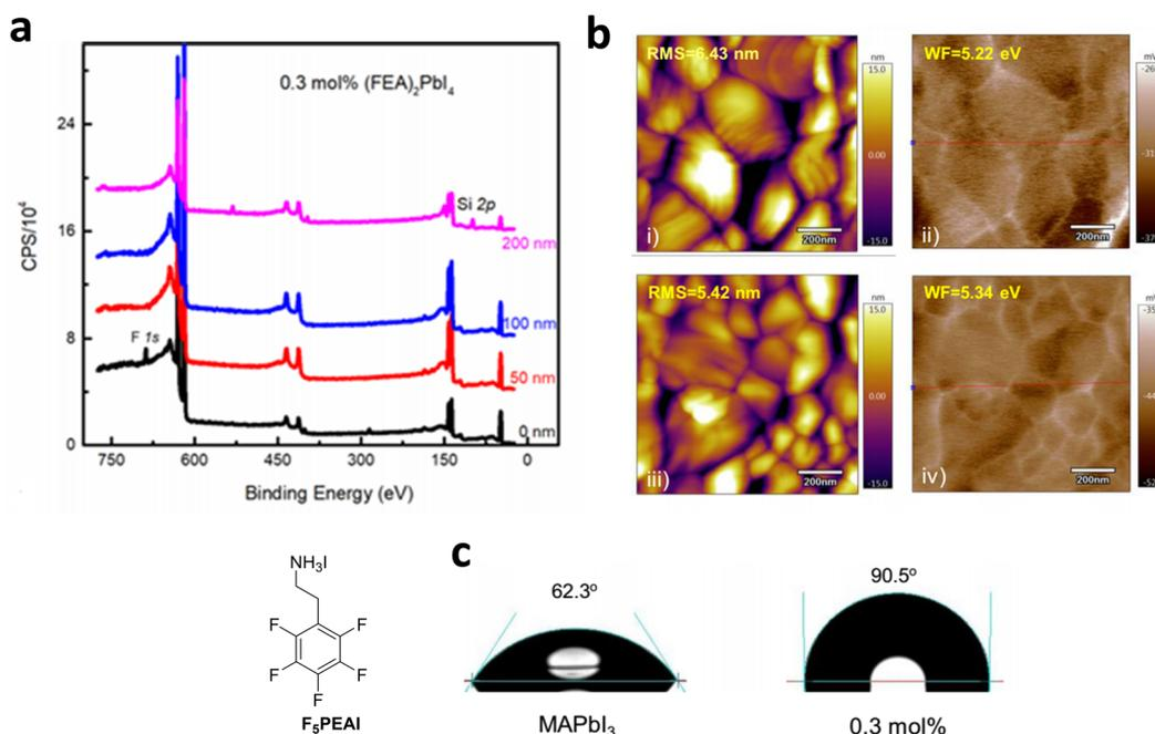
Fig. 27 (a) XPS-depth profiles of 0.3 mol% (F<sub>5</sub>PEA)<sub>2</sub>PbI<sub>4</sub> films. (b) AFM and SKPM images of MAPbI<sub>3</sub> (i and ii) and 0.3 mol% (F<sub>5</sub>PEA)<sub>2</sub>PbI<sub>4</sub> doped films (iii and iv). (c) Water contact angles of pristine and doped films.<sup>125</sup> Reproduced with permission from ref. 125. Copyright 2021, Springer Nature.
