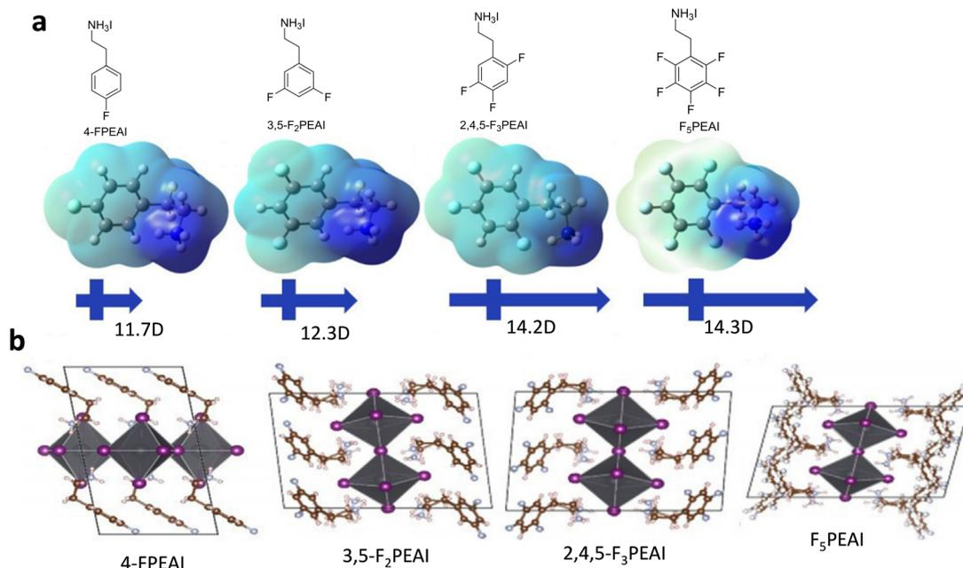
Fig. 21 (a) Dipole moments and ESPs (unit a.u.) of different fluorinated spacers. (b) The crystal structure of 2D-perovskites with different fluorinated cations, showing the enhanced lattice distortion with increasing numbers of fluorine atoms.<sup>35</sup> Reproduced with permission from ref. 35. Copyright 2022, Elsevier.
