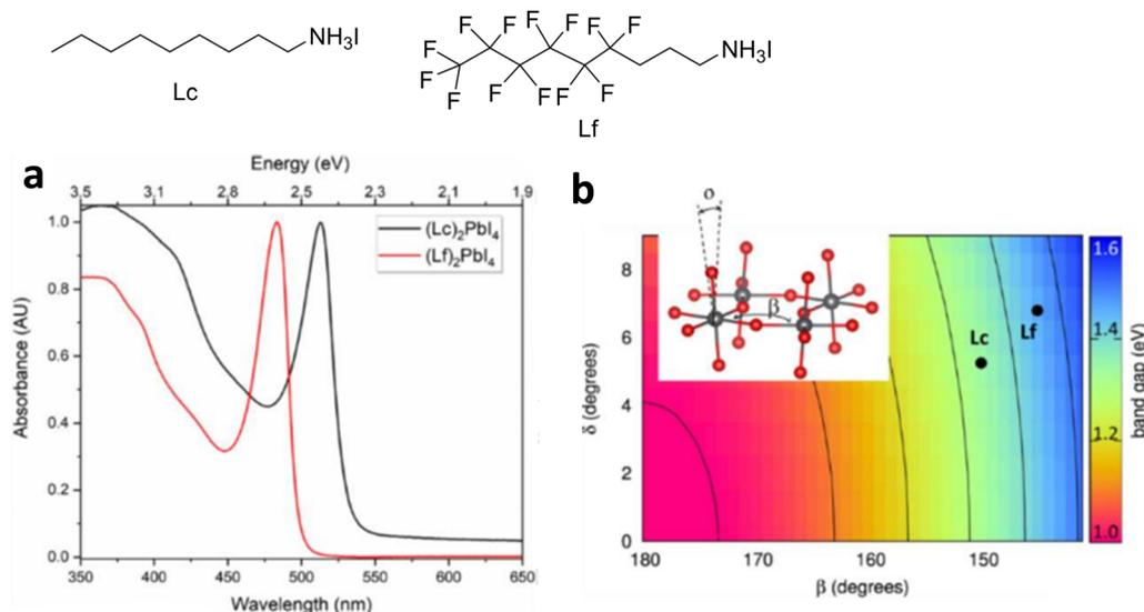
Fig. 8 (a) UV-Vis spectra of  $(\text{Lc})_2\text{PbI}_4$  and  $(\text{Lf})_2\text{PbI}_4$ . (b) Band gap map showing angles within and between the metal-halide octahedra.<sup>117</sup> Reproduced with permission from ref. 117. Copyright 2020, Frontiers Media S.A.
