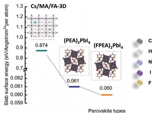
Fig. 19 The slab surface energy calculated for the Cs/MA/FA-triple cation 3D-perovskite,  $(\text{PEAI})_2\text{PbI}_4$  and  $(4\text{-FPEAI})_2\text{PbI}_4$ .<sup>57</sup> Reproduced with permission from ref. 57. Copyright 2019, John Wiley and Sons.
