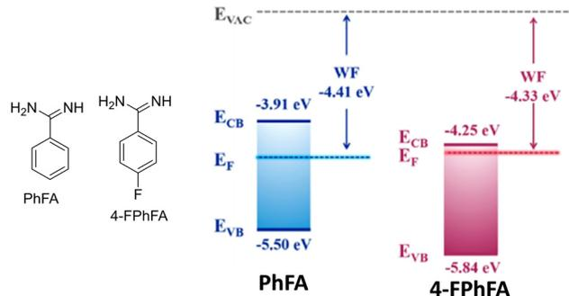
Fig. 16 The energy level diagrams for PhFA and 4-FPhFA-based perovskites, illustrating greater n-type character for the latter.<sup>59</sup> Reproduced with permission from ref. 59. Copyright 2021, American Chemical Society.
