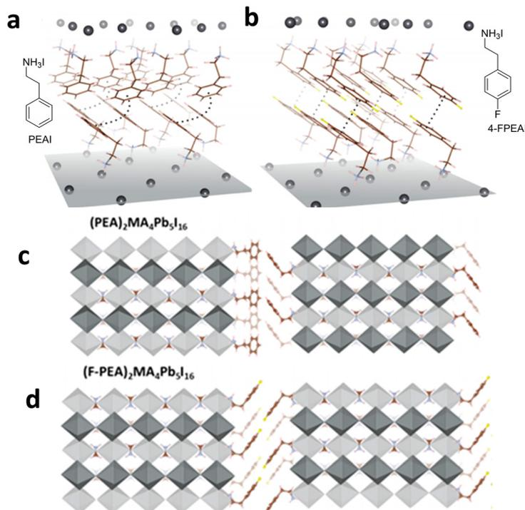
Fig. 7 (a and b) The crystal structure of  $(\text{PEA})_2\text{PbI}_4$  and  $(4\text{-FPEA})_2\text{PbI}_4$ . (c and d) The schematic crystal structures of RP-perovskites  $(\text{PEA})_2\text{MA}_4\text{Pb}_5\text{I}_{16}$  and  $(4\text{FPEA})_2\text{MA}_4\text{Pb}_5\text{I}_{16}$ .<sup>113</sup> Reproduced with permission from ref. 113. Copyright 2019, American Chemical Society.
