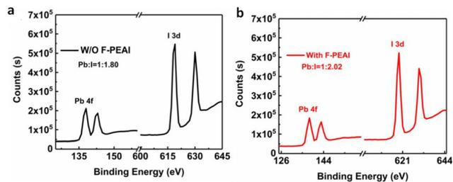
Fig. 26 (a) XPS profile of the control 3D-film showing the Pb:I ratio. (b) XPS spectrum of the passivated film showing an enhanced Pb:I ratio.<sup>11</sup> Reproduced with permission from ref. 11. Copyright 2021, American Chemical Society.
