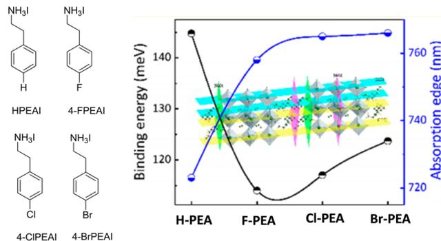
Fig. 12 The trend of binding energy and absorption edge across the series of RP-perovskites with PEA and different halogen-tethered PEA spacers.<sup>61</sup> Reproduced with permission from ref. 61. Copyright 2019, American Chemical Society.
