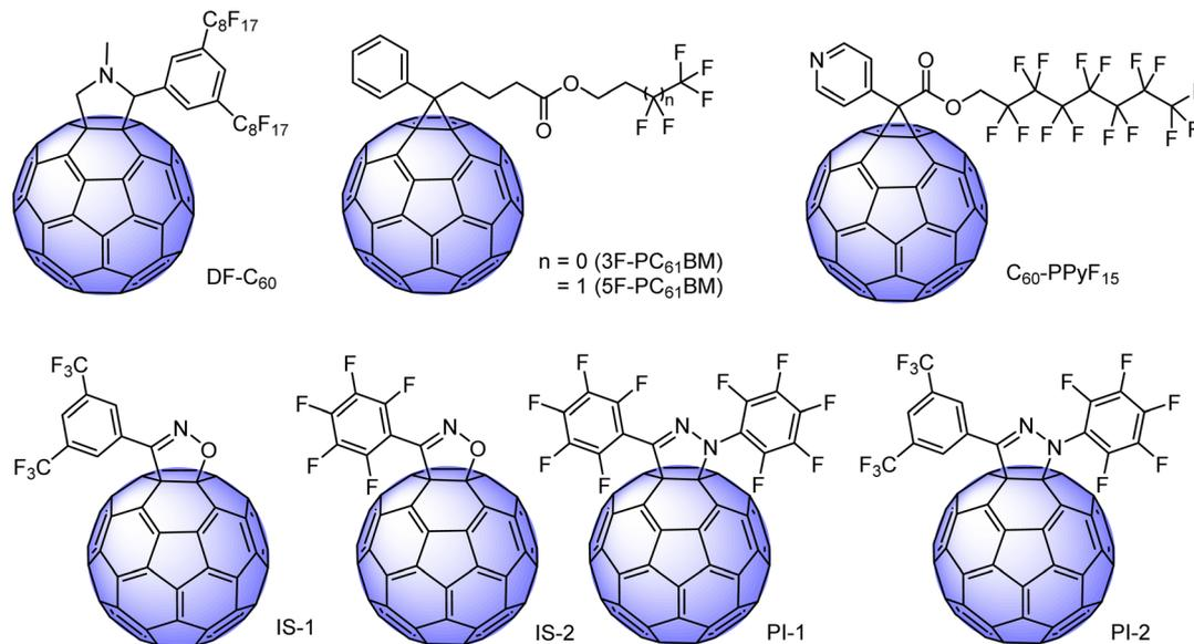
Fig. 32 Designs of fluorine-based fullerenes blended with perovskites for PV applications.<sup>132–136</sup>
