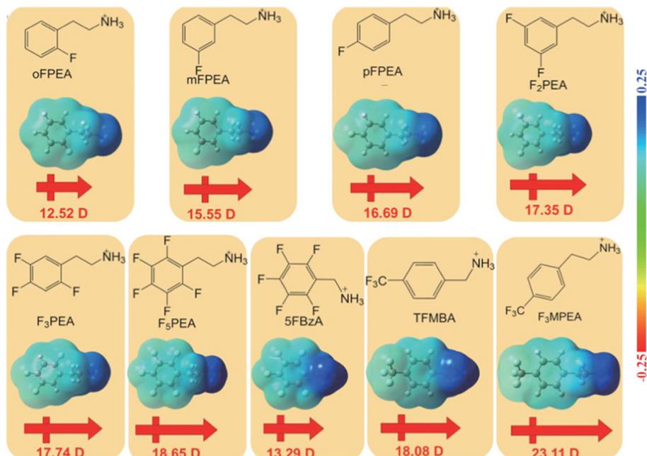
Fig. 1 Calculated dipole moments and electrostatic surface potentials (ESP) for different fluorinated spacers explored for developing perovskites (unit a.u.).<sup>100</sup> Reproduced with permission from ref. 100. Copyright 2022, IOPScience.
