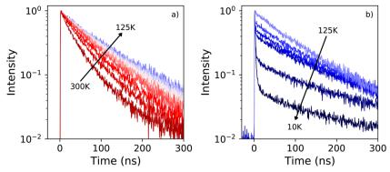
Fig. 6 (a) Temperature dependent X-ray excited decay spectra of PEA<sub>2</sub>PbBr<sub>4</sub> recorded from 125 K to 300 K, with a 25 K interval. The temperature decreases in the direction of the arrow. (b) Temperature dependent X-ray excited decay spectra of PEA<sub>2</sub>PbBr<sub>4</sub> recorded from 125 K to 25 K, with a 25 K interval, and at 10 K. The temperature decreases in the direction of the arrow
