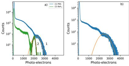
Fig. 8 Pulse height spectra recorded using a  $^{137}$ Cs  $\gamma$ -source and a PMT as detector (a) Small, similar sized, PEA<sub>2</sub>PbBr<sub>4</sub> and BaF<sub>2</sub>. (2 mm  $\times$  1 mm  $\times$ 0.3 mm) (b) Large PEA<sub>2</sub>PbBr<sub>4</sub> crystal (8 mm  $\times$  5 mm  $\times$  1 mm)
