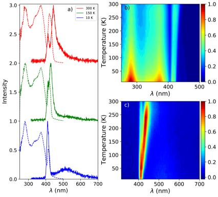
Fig. 1 (a) Temperature dependent photoluminescence emission ( $\lambda_{ex} = 260$  nm) and excitation ( $\lambda_{em} = 530$  nm) spectra of PEA<sub>2</sub>PbBr<sub>4</sub>, from top to bottom: 300 K, 150 K, and 10 K. (b) Temperature dependent photoluminescence excitation spectra ( $\lambda_{em}$  = 530 nm), from 300 K down to 10 K. (c) Temperature dependent photoluminescence emission spectra ( $\lambda_{ex}$  = 260 nm), from 300 K down to 10 K.
