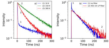
Fig. 5 (a) Temperature dependent X-ray excited decay spectra of  $PEA_2PbBr_4$  recorded at 10 K, 75 K, and 300 K. (b) X-ray excited decay spectra of  $PEA_2PbBr_4$  recorded at 10 K with and without 455 nm long pas filter.
