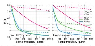
Fig. 5  $\,$  MTF  $_{tot}$  (solid lines) and MTF  $_{scint}$  (dashed lines) for 5  $\mu m$  films supported by 150  $\mu$ m substrates, evaluated for NA = 0.80 at different X-ray energies. The corresponding SCF, substrate and X-ray energies selected for the simulations are indicated in the figure
