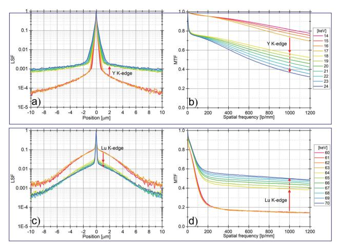
Fig. 3 Simulated LSFs (left) and MTFs (right) for a 5 μm LAG:Ce SCF supported by 150 μm YAG substrate. (a and b) X-ray energies from 14 to 24 keV. K-edge energy of Y is 17.04 keV. (c and d) X-ray energies from 60-70 keV. K-edge of Lu is 63.3 keV.
