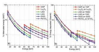
Fig. 2 (a) Percentage of the incident beam energy attenuated by various kinds of 5  $\mu$ m thick SCFs, calculated using data from the NIST database.<sup>32</sup> (b) Percentage of the incident beam energy deposited in various 5  $\mu m$  SCFs supported by 150  $\mu m$  substrates, calculated by tracking all the secondary X-rays and electrons using our application based on the Monte Carlo
