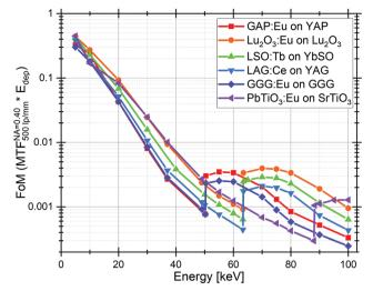
Fig. 6 The proposed figure of merit (FoM) calculated from the contrast in the MTF blurred by optics (NA = 0.40) at 500 lp mm $^{-1}$  and the energy deposited in the SCF. Values are extracted from simulations at X-ray energies from 5-100 keV for 5 μm SCFs supported by 150 μm substrates.
