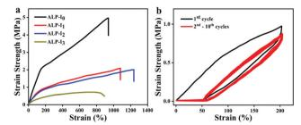
Fig. 3 Mechanical properties of ionogel: (a) the tensile stress-strain curves of the ionogel with different IL addition; (b) 10 times repeated
