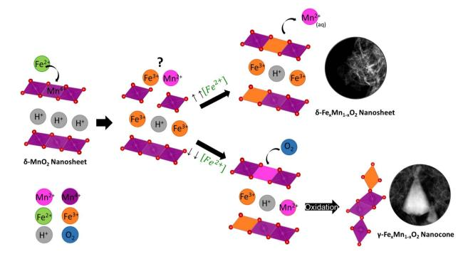
Schematic mechanism governing the synthesis of  $Fe_vMn_{1-x}O_2$  nanosheets and nanocones through galvanic exchange reaction.
