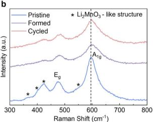
Fig. 4 Solid state NMR and Raman analysis. (a) <sup>7</sup>Li MAS ssNMR MAT-PASS spectra of the Formed and Cycled samples and (b) Raman spectra of the Pristine, Formed and Cycled samples. All measurements are taken under an inert gas atmosphere. Pertinent peaks are assigned.
