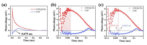
Fig. 7 (a) The transient photovoltage curves, the corresponding (b) amount of charge extraction and (c) maximum charge extraction time of the COF and COF@CDs.
