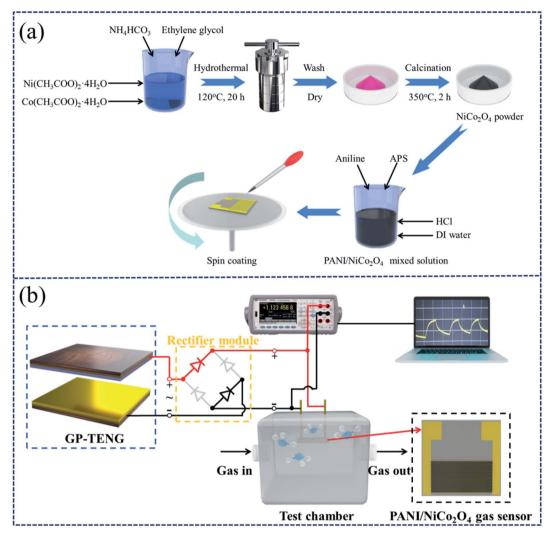
Fig. 2 (a) The diagram of preparation process of the NH<sub>3</sub> gas sensor based on the PANI/NiCo<sub>2</sub>O<sub>4</sub> composite. (b) The experimental test platform of the self-powered GPAS based on the PANI/NiCo<sub>2</sub>O<sub>4</sub> composite.
