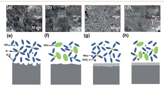
Fig. 3 SEM images of aluminum anodes in (a) blank, (b) 8 M KOAc, (c)  $0.02 \text{ M Na}_2\text{SnO}_3$  and (d) HHCE after 3 h of immersion. Schematic illustrations of the corrosion behavior of aluminum anodes in (e) blank, (f) 8 M KOAc, (g)  $0.02 \text{ M Na}_2\text{SnO}_3$  and (h) HHCE.
