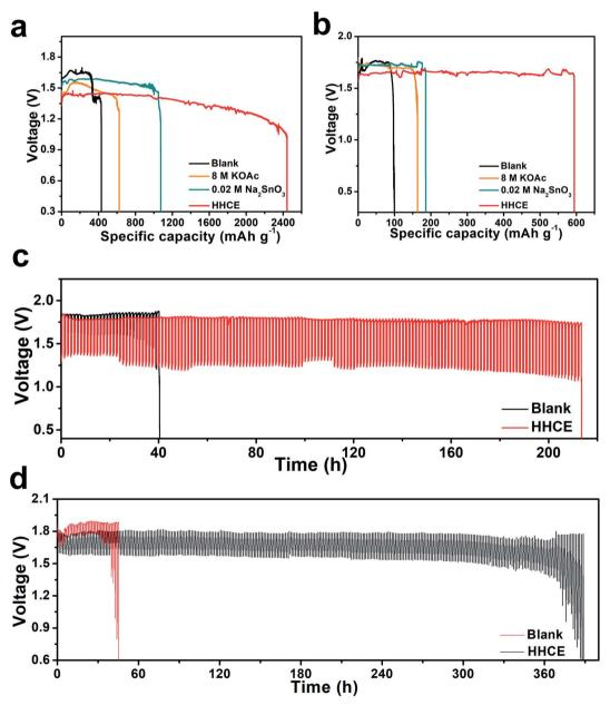
Fig. 5 Galvanostatic discharge curves of full batteries with different electrolytes at a current density of (a) 25 mA cm<sup>-2</sup>, and (b) 5 mA cm<sup>-2</sup>. Voltage *versus* time plots for on/off cycling of the full batteries at a current density of (c) 25 mA cm<sup>-2</sup>, and (d) 5 mA cm<sup>-2</sup>.
