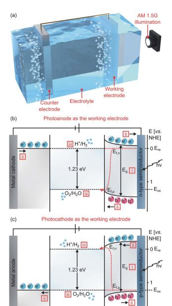
Fig. 3 (a) An artist's rendition of a basic PEC water splitting components comprising of a working electrode and a counter electrode immersed in an electrolyte with AM 1.5G illumination as a light source. Three steps of overall PEC water splitting in (b) photoanode and (c) photocathode: (i)  $E_q$  excitation, (ii) charge separation and transfer, (iii) surface reactions of OER and HER
