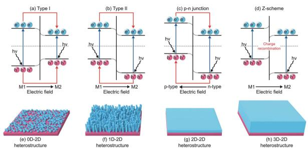
Fig. 6 Possible (a–d) charge transfer mechanisms throughout the heterostructure interface areas and (e–h) different types of heterostructures with various mixed-dimensionality. In panel (a–d), M1 and M2 are material 1 and material 2, respectively, while the blue and red lines represent band gap excitation and charge transfer at the interface, respectively.
