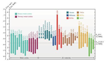
Fig. 5 Representative Eq and band positions of MOs and 2D materials. Upper and lower horizontal dashed lines represent Ere of 0 V vs. NHE and  $E_{\rm ox}$  of 1.23 V vs. NHE, respectively
