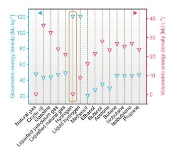
Fig. 1 Gravimetric and volumetric energy densities of various fuels based on the lower heating value (LHV). Data is adapted from ref. 7.
