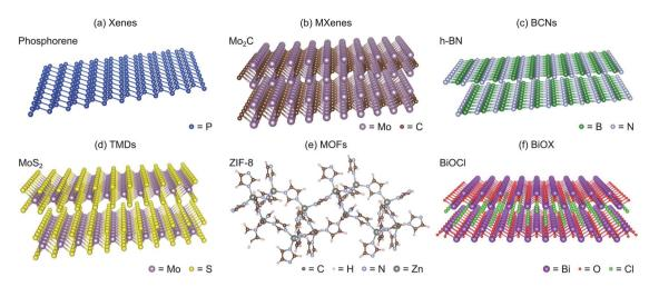
Fig. 4 Representative 2D materials family categorized by their compositions. (a) Phosphorene of Xenes, (b) Mo<sub>2</sub>C of MXenes, (c) h-BN of boron carbon nitrides (BCNs), (d) MoS<sub>2</sub> of transition metal dichalcogenides (TMDs), (e) ZIF-8 of metal-organic frameworks (MOFs), and (f) BiOCl of bismuth oxyhalides (BiOX).
