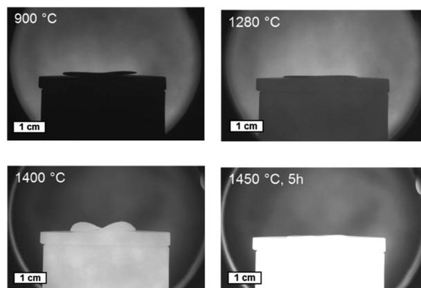
Fig. 7 Sintering behaviour of a bi-layer assembly of BZCY-NiO/BZCY-SU at different temperatures captured in an optical dilatometer.
