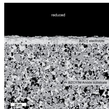
Fig. 11 SEM cross sections of final sintered BZCY–NiO/BZCY bi-layer assemblies at 1500 °C for 6 h. (a) Unreduced, (b) reduced in Ar/H<sub>2</sub> at 900 °C.
