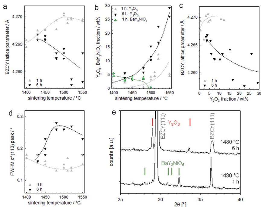
Fig. 14 XRD results for the assemblies of Fig. 13. (a) Lattice parameter of the BZCY perovskite, (b) fraction of  $\text{Y}_2\text{O}_3$  and  $\text{BaY}_2\text{NiO}_5$  second phases, (c) relation of BZCY lattice parameter and  $\text{Y}_2\text{O}_3$  fraction, (d) full width at half maximum of the (110) peak of the BZCY, (e) diffractograms for samples sintered for 1 h and 6 h at 1480 °C with  $\text{Y}_2\text{O}_3$  and  $\text{BaY}_2\text{NiO}_5$  peaks indicated.
