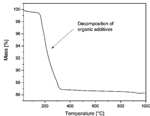
Fig. 4 Thermogravimetric measurement of NiO/BZCY green tapes in air, heating rate of 5 K min<sup>-1</sup>.
