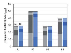
Fig. 7 Breakdown of the equipment costs of routes P1-P4 (a) by synthesis steps, left grey column from bottom to top: MeOH, FA (aqueous or anhydrous), OME<sub>3-5</sub>, heat recovery, and OME<sub>1</sub> (only P3 and P4) and (b) by equipment type, right blue column from bottom to top: compressors, heat exchangers, reactors, and separators. The marginal contribution of pump costs is not visible in this diagram.
