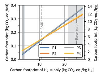
Fig. 15 Carbon footprint of all four OME<sub>3-5</sub> process routes as a function of the carbon footprint of H<sub>2</sub> supply. The left y-axis shows the carbon footprint in kg CO<sub>2</sub>-eq. per MJ, while the right y-axis additionally indicates the results in kg  ${\rm CO_2\text{-}eq.}$  per  ${\rm l_{DE}}.$  The shaded areas indicate the carbon footprint ranges of H<sub>2</sub> supply for the years 2018 (light grey) and 2050 (dark grey).68 SMR: steam methane reforming.
