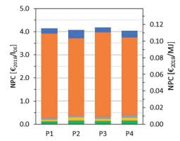
Fig. 9 Breakdown of net production costs (NPC) of routes P1-P4:  $\blacksquare$  ACC',  $\blacksquare$  OPEX'<sub>R&U</sub>,  $\blacksquare$  C'<sub>labor</sub>,  $\blacksquare$  OPEX'<sub>dir</sub>, and  $\blacksquare$  OPEX'<sub>ind</sub>.
