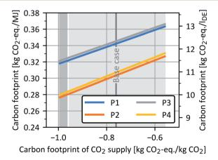
Fig. 14 Carbon footprint of all four OME<sub>3-5</sub> process routes as a function of the carbon footprint of CO<sub>2</sub> supply. The left y-axis shows the carbon footprint in kg  $CO_2$ -eq. per MJ, while the right y-axis additionally indicates results in kg CO<sub>2</sub>-eq. per l<sub>DE</sub>. The shaded areas indicate the carbon footprint ranges of CO2 supply from DAC (light grey) and MEA cement (dark grey) for the years 2018 and 2050.68
