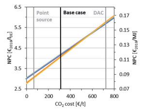
Fig. 10 Dependence of NPC on the CO<sub>2</sub> cost: — P1, — P2, — P3 and P4. Point source cost from ref. 69 and DAC cost from ref. 70. All other raw material costs are fixed as in the base case.
