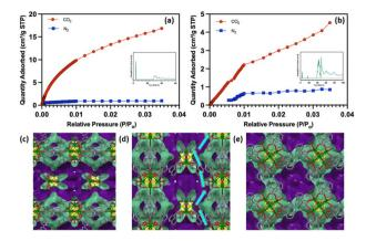
Fig. 7 Adsorption isotherms for (a) Y-BCA-3D and (b) Y-BCA-2D. Representation of sinusoidal voids/channels (purple) in Y-BCA-3D (c) viewed along a-axis, (d) viewed along b-axis and gas passage is highlighted by arrows, and (e) viewed along c-axis show presence of deep spherical cavities with a diameter of 6.3 Å.
