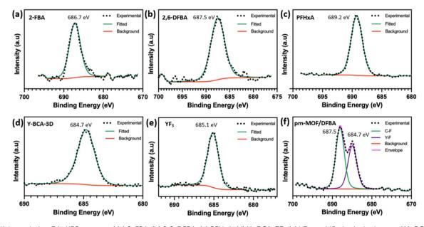
Fig. 6 High resolution F 1s XPS spectra of (a) 2-FBA, (b) 2,6-DFBA, (c) PFHxA, (d) Y-BCA-3D, (e) YF<sub>3</sub>, and (f) physical mixture of Y-BCA-3D and 2,6-DFBA.
