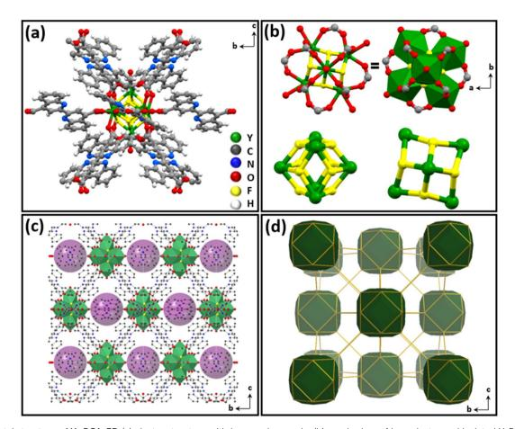
Fig. 4 Crystal structure of Y-BCA-3D (a) cluster structure with hexanuclear node, (b) c-axis view of hexacluster and isolated  $Y_6F_8$  cluster, (c) extended 3D network view along the a-axis showing 6.3 Å spherical cavities (purple), and (d) underlying net topology of the MOF viewed along the a-axis.
