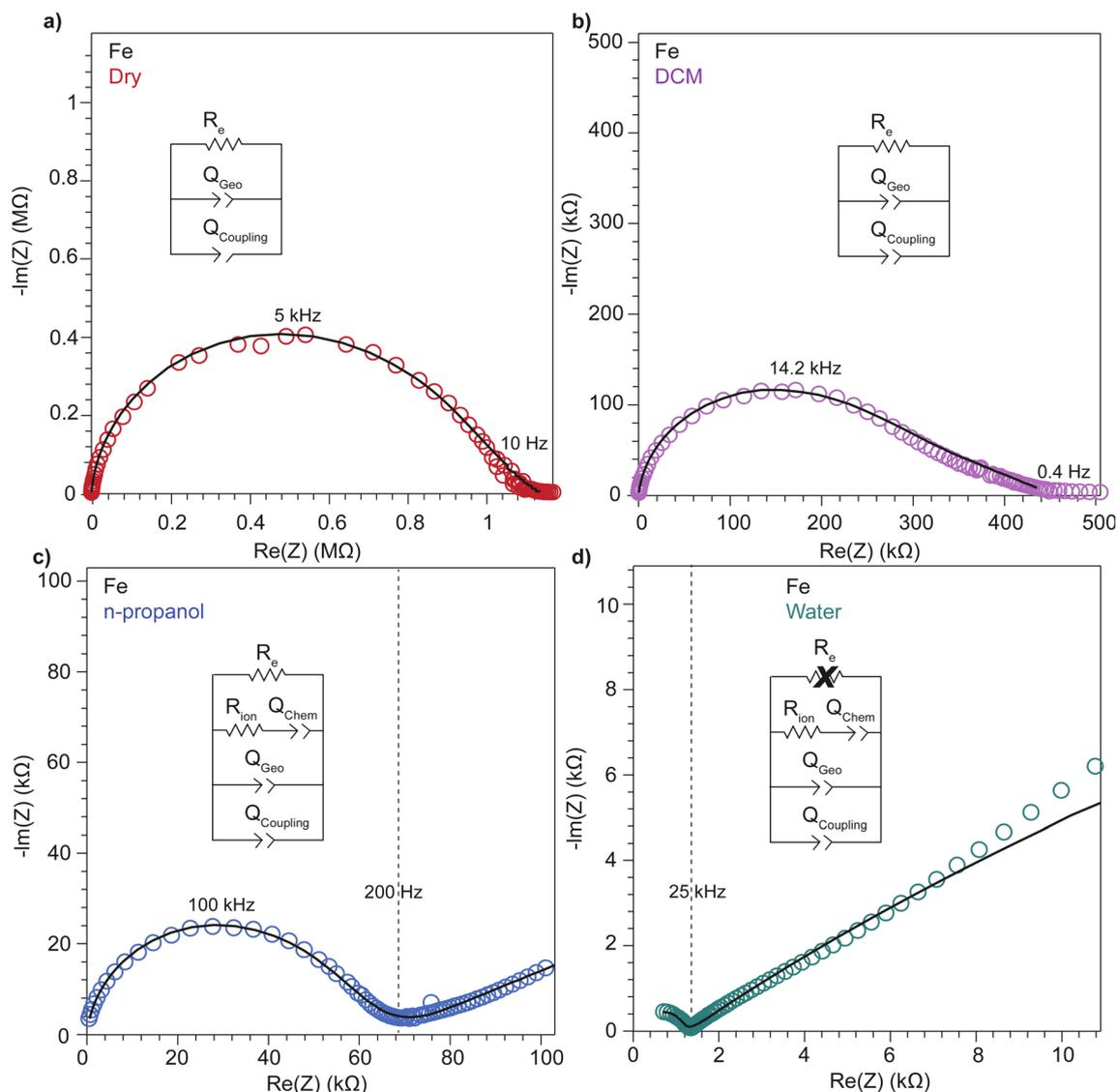
Fig. 3 Nyquist plots of  $\text{TMA}_2\text{FeGe}_4\text{S}_{10}$  pressed-pellets when dry (a) and after addition of DCM (b), *n*-propanol (c), and deionized water (d). Black traces represent fits to the equivalent circuit diagrams shown in the figure. Crossed-out circuit elements denote elements that are too large to adequately fit to the impedance response.
