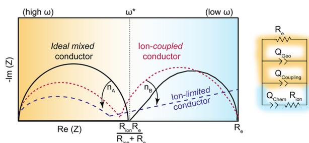
Scheme 3 Generalized impedance response for an ideal mixed conductor (black solid trace), an ion-coupled conductor (dotted red trace;  $\text{TMA}_2\text{ZnGe}_4\text{S}_{10}$ ), and ion-limited conductor (dotted blue trace;  $\text{TMA}_2\text{FeGe}_4\text{S}_{10}$ ).
