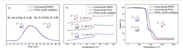
Fig. 4 Characterization of PVAc 5a prepared by exhaustive BV post-modification of PMVK 3a. Comparison of (a) SEC, (b) DSC, and (c) TGA data of PMVK 3a, commercial PVAc and PVAc 5a obtained by BV oxidation.
