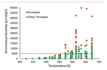
Fig. 5 Scatter plot showing the ammonia productivities of various heterogeneous catalysts as a function of temperature for ammonia synthesis at pressures no greater than 10 bar. The same catalyst systems were represented in terms of their efficiency in Fig. 4. References for activity data of the individual catalyst systems can be found in Table 1.
