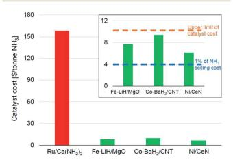
Fig. 6 Catalyst costs per tonne of ammonia produced assuming a catalyst lifetime of 6 months. The catalyst activity data was taken from the following references: Ru/Ca(NH<sub>2</sub>)<sub>2</sub>, $^{70}$  Fe–LiH/MgO, $^{112}$  Co–BaH<sub>2</sub>/CNT, $^{99}$  and Ni/CeN. $^{86}$  The cost of the materials per kg were taken as \$400, \$8, \$15 and \$10 respectively, which are assumed from current element costs $^{125}$  and previously reported costs of similar materials. $^{17}$
