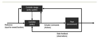
Fig. 5 Reinforcement learning can be described<sup>30</sup> as a method to tune, enhance or substitute traditional control systems.
