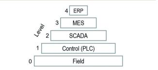
Fig. 6 Simplified hierarchical view of automation infrastructures in the standard ANSI/ISA-95
