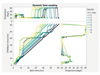
Fig. 22 A comparison between the (original) batch time vs. time dynamically warped shows the rate at which the batches are progressing relative to the reference (batchID 1). In this illustrative example, batches are getting shorter so the rate is always positive.
