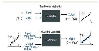
Fig. 1 Contrary to the traditional approach, where first principles models are used, machine learning fits empirical models using experimental data (training data). A proper data split is necessary to introduce the right amount of model complexity and avoid overfitting.
