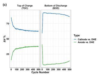
Fig. 6 (a) OCV, (b) overpotentials ( $\Delta V$ ), and (c) the relative proportion of overpotential, at the top of charge (TOC) and bottom of discharge (BOD) as a function of cycle numbers for the full cell and individual electrode (cathode or anode vs. DHE). For (a), the purple line is the difference of OCV between cathode and anode. For (b), the purple line is the sum of overpotential of individual electrodes (cathode + anode).
