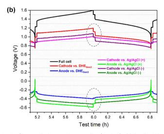
**Fig. 3** Charge-discharge voltage profiles (vs. time) of full cell and its individual electrode (cathode or anode) vs. RE (DHE, Ag/AgCl (+) or Ag/AgCl (-)) of a scaled vanadium redox flow battery (49 cm² in active area): (a) for the initial 10 cycles, and (b) for the 2nd cycle, enlarged area highlighted in (a). Ag/AgCl (+) and Ag/AgCl (-) are the Ag/AgCl reference electrodes that are in the inlet of catholyte and anolyte respectively.
