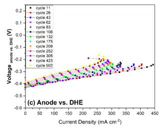
Fig. 7 Polarization curves as a function of cycle numbers for (a) full cell, (b) cathode vs. DHE, and (c) anode vs. DHE.
