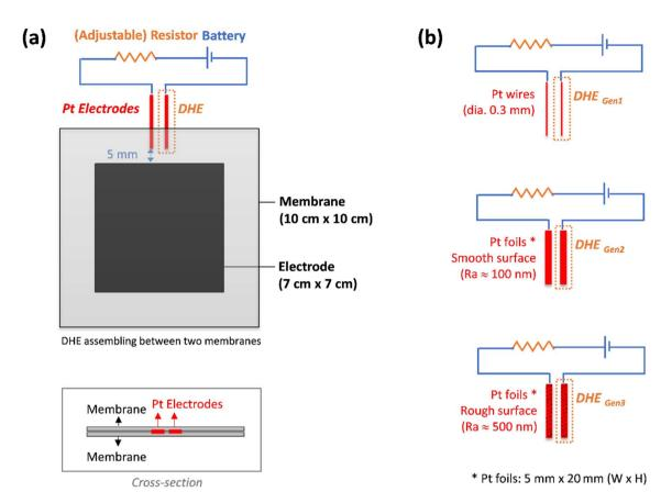
Fig. 1 (a) A scheme of detailed design of DHE in an all-vanadium redox flow battery, and (b) DHE with three types of Pt electrodes: Pt wires  $(DHE_{Gen1})$ , Pt foils with smooth surface  $(DHE_{Gen2})$ , and Pt foils with rough surface  $(DHE_{Gen3})$ .
