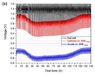
Fig. 2 Charge–discharge voltage profiles (vs. time) of full cell (cathode vs. anode) and its individual electrode (cathode or anode) vs. DHE (with different Pt electrodes-based design) during long-term cycling of a scaled vanadium redox flow battery (49 cm² in active area): (a) DHE\_Gen1 (w/ Pt wires), (b) DHE\_Gen2 (w/ Pt foils of smooth surface), and (c) DHE\_Gen3 (w/ Pt foils of rough surface).
