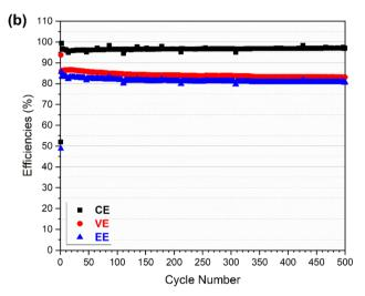
Fig. 4 Cell performances of an all-vanadium RFB using GfE commercial electrolyte with V  $(1.6\ M)$  and N212 double membranes: (a) charge and discharge capacities as a function of cycle number; and (b) coulombic efficiency (CE), voltage efficiency (VE), and energy efficiency (EE) as a function of cycle number.
