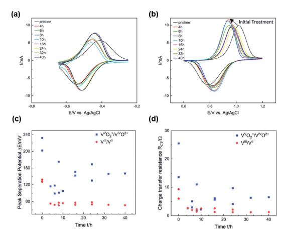
Fig. 3 Electrocatalytic activity of thermally activated GF. (a and b) CV curves recorded in the (a) negative and (b) positive half-cell. (c) Peak separation potential in the negative and positive half-cell. (d) EIS at an applied potential in the negative and positive half-cell.
