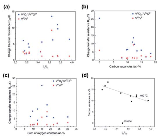
Fig. 5 Structure—activity correlation of thermally activated GF. Correlation between (a)  $R_{CT}$  and defect type, (b)  $R_{CT}$  and  $C_V$ , (c)  $R_{CT}$  and oxygen concentration, (d)  $C_V$  and defect type.
