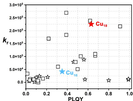
**Fig. 1** Summary of calculated radiative decay rate ( $k_r = \Phi/\tau$ ) versus PLQY ( $\Phi$ ) of all reported atomically precise CuNCs, including protected  $\text{S}^-$ ,  $\text{P}^-$  and  $\text{I}$  ligands (squares) and  $\text{C}\equiv\text{C}^-$  (pentagons) (see Table S5† for details).
