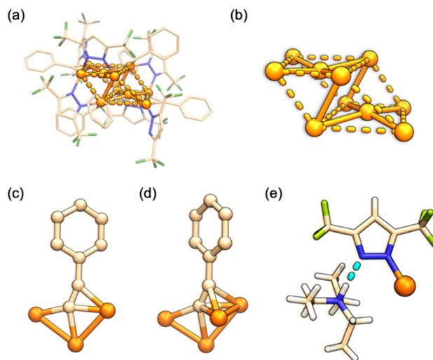
**Fig. 2** The crystal structure of **Cu<sub>10</sub>** (only structures of **Cu<sub>10</sub>-a** are shown for clarity). (a) Overall structure; (b) metal core and (c) and (d) ligation modes of an alkyne and (e) the monodentate mode and hydrogen bonding of Pz<sup>–</sup>.
