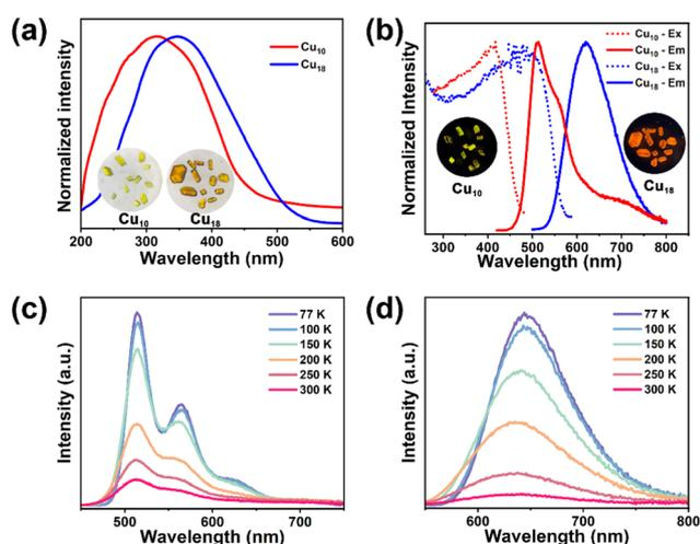
**Fig. 4** Solid-state UV-Vis absorption (a), and excitation and emission spectra (b) of crystalline powders of **Cu<sub>10</sub>** and **Cu<sub>18</sub>**. Insets are **Cu<sub>10</sub>** and **Cu<sub>18</sub>** irradiated by ambient light and a hand-held UV lamp. Temperature-dependent emission spectra of **Cu<sub>10</sub>** at  $\lambda_{ex} = 420$  nm (c) and **Cu<sub>18</sub>** at  $\lambda_{ex} = 500$  nm (d).
