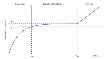
Fig. 1 Schematic of a typical hydrate formation profile through guest gas consumption. Here,  $n_{\text{sat}}$  is the molar saturation value that occurs at  $t_{\text{sat}}$  and  $n_{\text{liq}}$  is the final number of moles in the supersaturated solution at nucleation, which occurs at  $t_{\text{nuc}}$ .
