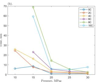
Fig. 7 The time required for the 1 ppm O-MWCNT-methane-water system to reach (a) 200 mPa s and (b) 500 mPa s from the onset of hydrate formation at various pressures.
