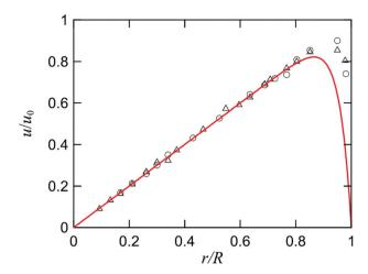
Fig. 37 The distribution of azimuthal velocity  $u/u_0$  of the ferrofluid surface in a cylinder of R = 2.33 cm, angular velocity 60 Hz. The symbols mark the experimental data:  $\bigcirc -H = 100 \text{ Oe}$ ,  $\triangle -H = 200 \text{ Oe}$ ,  $^{613}$  and the solid line is for the theoretical values found by Shliomis (reproduced from ref. 623 with permission from Am. Phys. Soc., copyright 2021).
