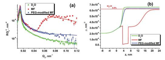
Fig. 21 (a) Experimental reflectivity curves (Fresnel representation) together with fits (solid lines) for pure D<sub>2</sub>O (green squares), initial aqueous MF (red circles) and PEG-modified MF (blue triangles); (b) found from experimental data SLD profiles for three studied kinds of solid/liquid interfaces. The calculated mean SLD for the initial ferrofluid (concentration 0.8%) is shown (dashed line) for comparison (reproduced from ref. 366 with permission from Elsevier, copyright 2017).
